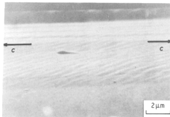
Figure 9 The characteristic pyramidal plane slip traces at approximately 18^\circ to the c -axis.
